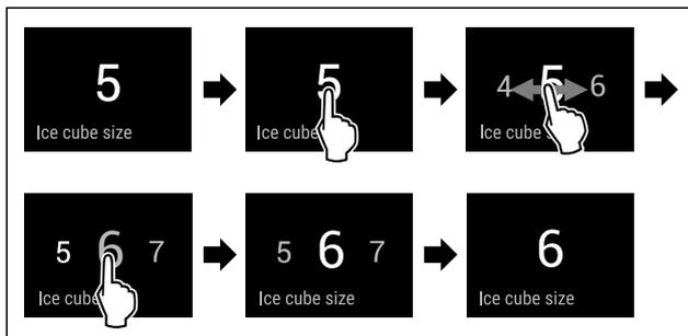
Fig. 62 Example illustration: Switch from value 5 to value 6.
