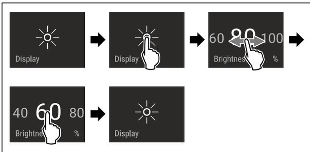
Fig. 67 Example illustration: Switch from 80 % to 60 %.
